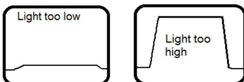
**Measurement data:** The tester measures the time that the waveform is flat and stable; this is the time that the shutter is fully open. If you have a waveform that is not stable you will get an inaccurate time measurement.
